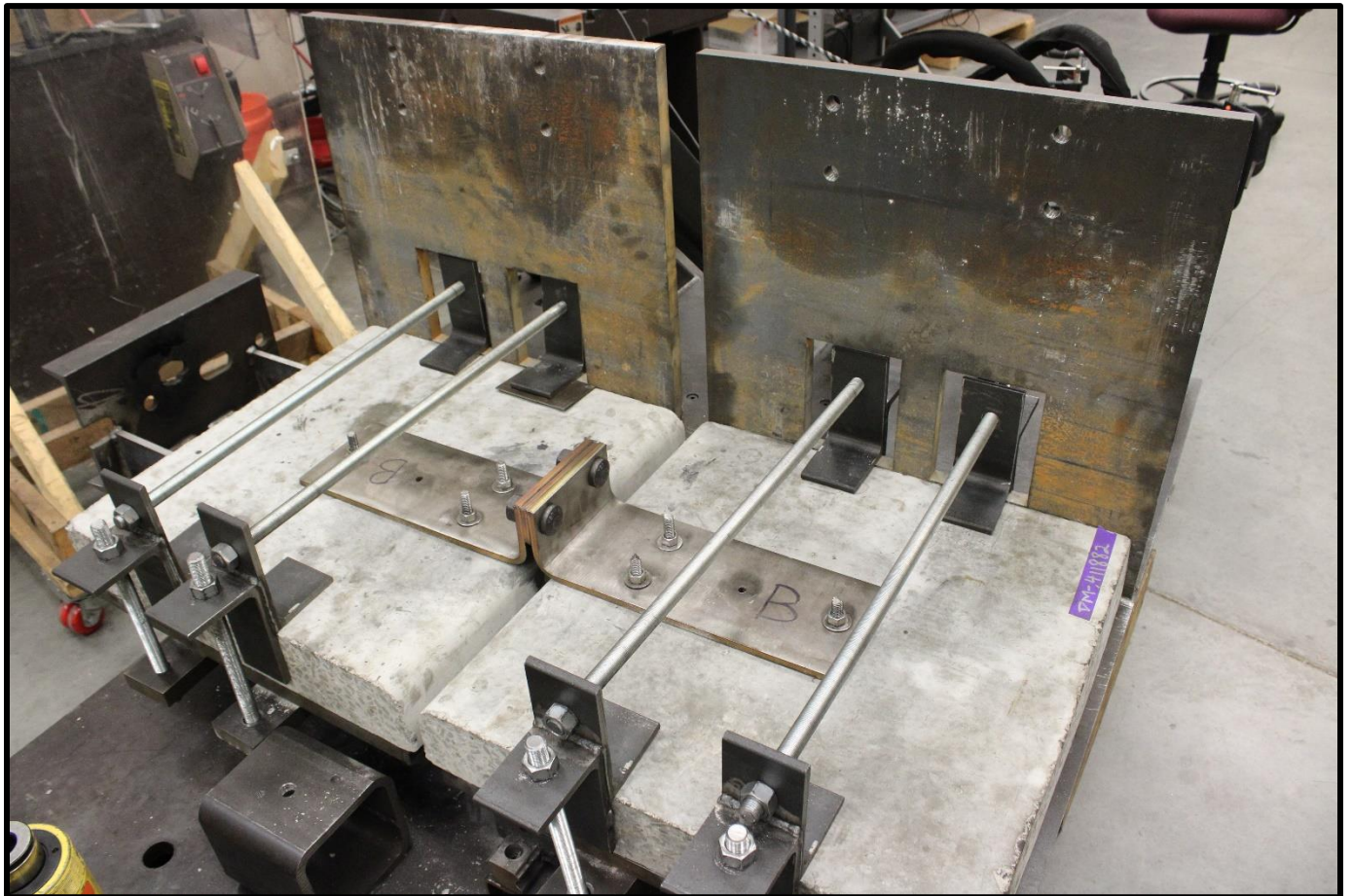
Figure 11: Bracket B - In-Plane Shear Test configuration
