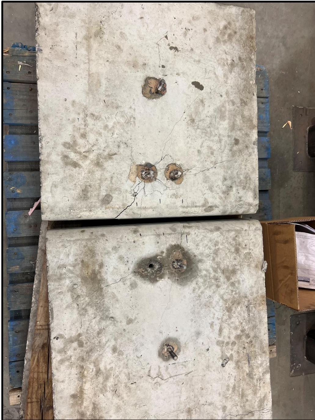
Figure 12: Visible crack formation on the concrete slabs after bringing Bracket B to 10,000 lbf during In-Plane Shear Test
