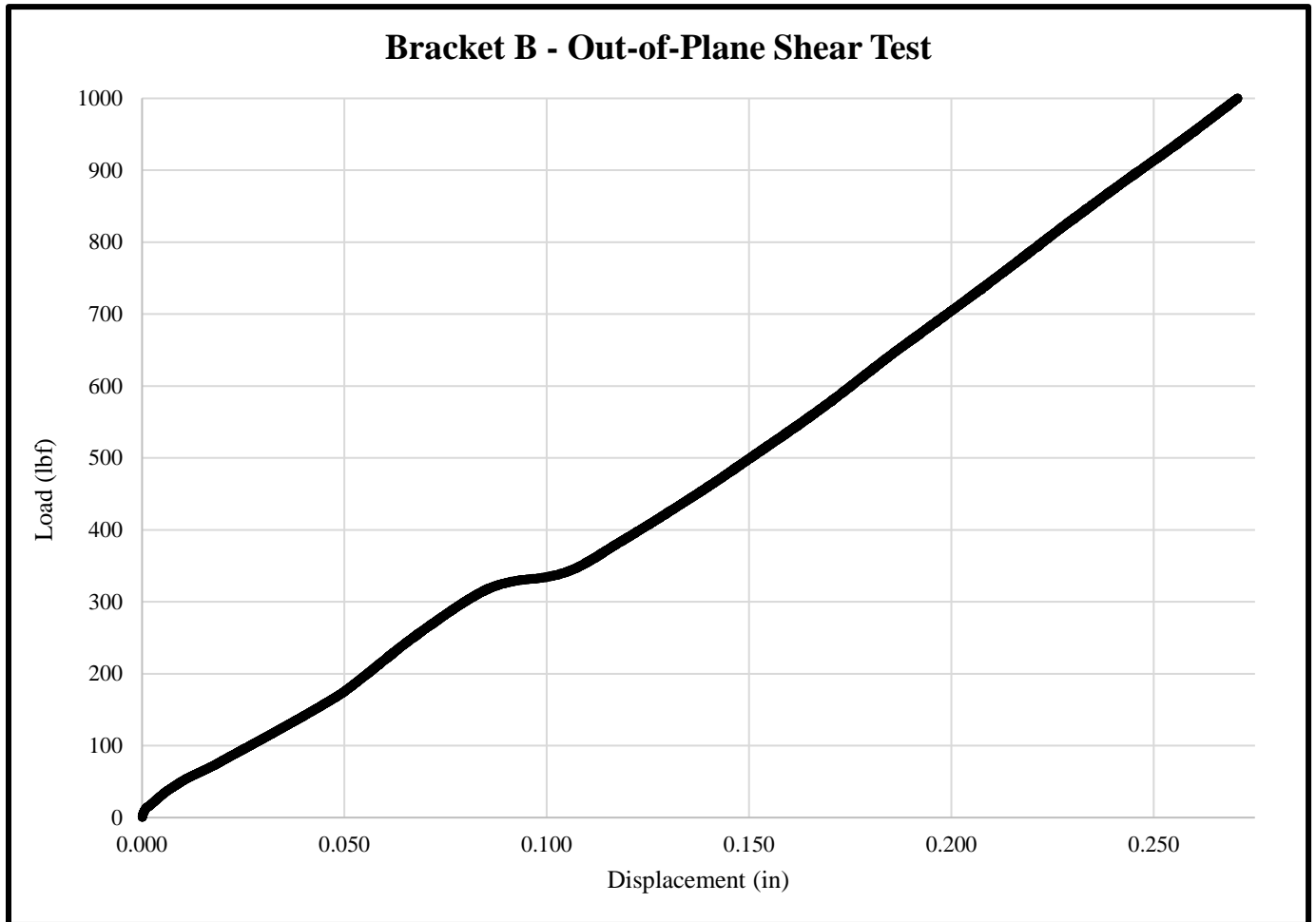
Figure 18: Bracket B - Out-of-Plane Shear data acquisition
